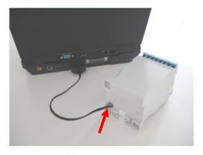
Connect the RJ11 modular plug of the cable to the PROG connection located at the rear side of the SELCO G-Line relay or the front of T7900. You will need to depress the small plastic tab in order to make the plug "snap" into the connector.
